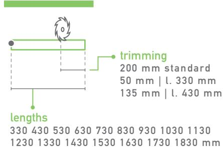
**EN** One of the all-time CCE classics, available with many different combination of seals and plungers, it guarantees a high efficiency. Its mechanism can be pulled out from both hinge and lock sides (CCE patent). This model can be installed also on pivoting doors in combination with Actuator Pivot accessory.
